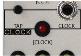
**Internal Clock** - The internal Midi 3 clock utilizes the TAP tempo button to modify the rate of the internal clock. 2 or 3 taps are needed to determine the internal clock tempo.
