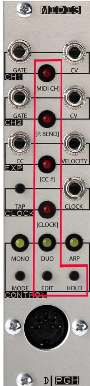
**EDIT MIDI CHANNEL** - The MIDI CH parameter assigns the midi channel. Pressing the HOLD button cycles through available options. Respond to all channels followed by channel 1 through channel 16. The number of times the LED blinks corresponds to the selected midi channel: 1 blink for channel 1, 2 for channel 2, etc... For all channels, the LED will blink at a steady rate.
