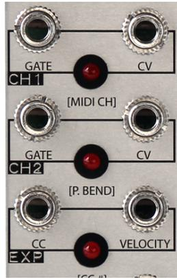
**Channel 1 Gate Out** - Channel 1 gate outputs a signal of either 0v (off) or 5v (on). This signal can be used to trigger an envelope generator, sequencer, logic module, or any other module that requires a gate input. The Channel 1 Gate is active when the Channel 1 LED is lit.
